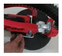
Telescopic pipe installation (Insert the telescopic pipe into the front pipe, adjust to the desired length, turn the locking nut into the front plastic pipe and lock.)
